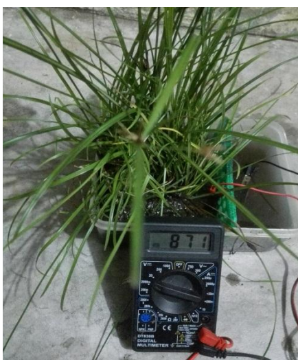
Figure 3 Experimental Setup of the double chambered P-MFC.
