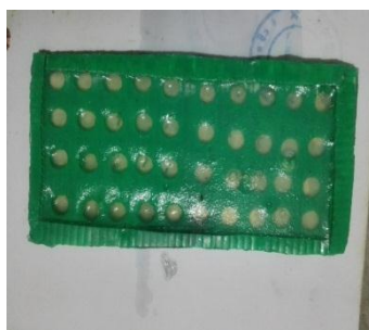
Figure 4 Agar gelatin Salt Bridge for the proton exchange membrane.
